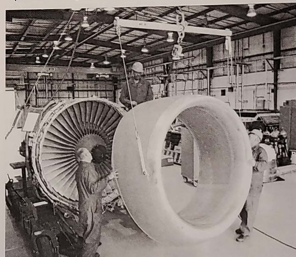
Master Sgts. Keith Brown, Floyd Gordon and Wayne Miller remove the nose cowl from the old engine as part of the QEC (quick engine change) process.
