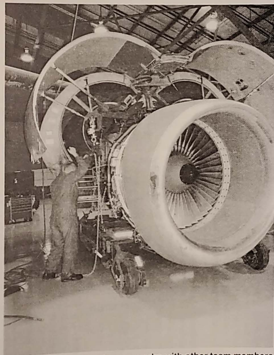
Tech Sgt. Daniel Anderson works with other team members to position the engine under the strut to raise the engine in place. The entire process takes approximately five hours.
